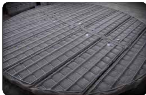
5- Two phase separators (Mist eliminator for Aria Sasol Polymer Co.)
