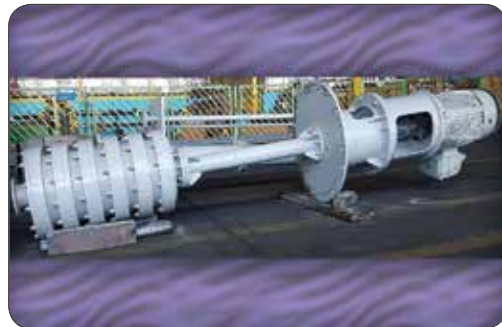
ESFAHAN Refinery Pump Model: VDL6-40.250 Capacity: 14 m 3 /h, Head: 127 m, Power: 30 KW
