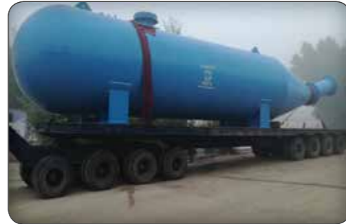
Surge Tank – Persian Gulf Water Transmission – WAS Co.
