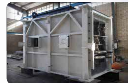
Fired Heaters (Manufacturing of Fired heaters for Bushehr Petrochemical Company)
