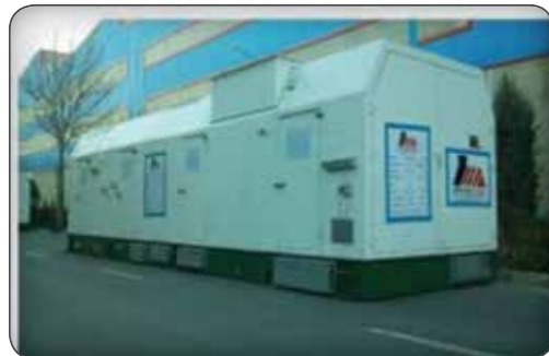
Construction of Acoustic Enclosure units for Industrial 25MW Turbo Compressor Turbines (Engineering & Manufacturing Company (TUGA)).
