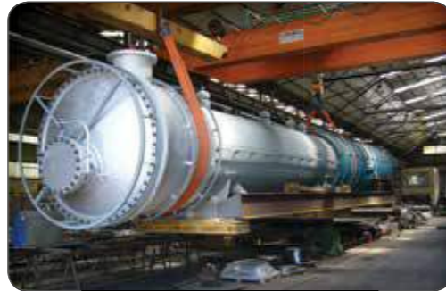
Waste Heat Boiler
