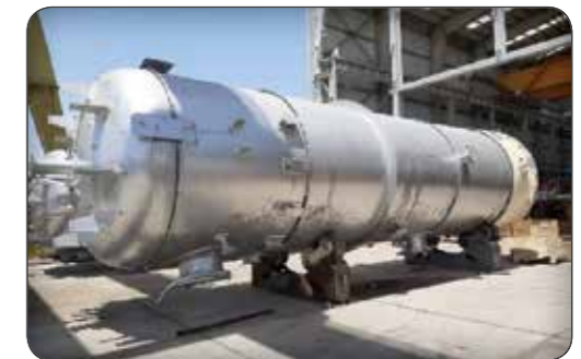
Separators: Vertical and Horizontal Design With Attachments, Including Internals, Ladder, Platform, External Jacket, Internal
