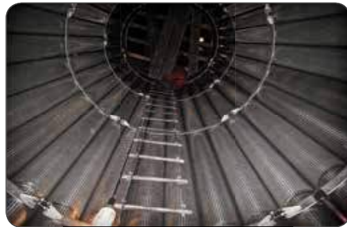
1- All types of Reactor Internals (CCR reactor of Persian Gulf Star Refinery)
