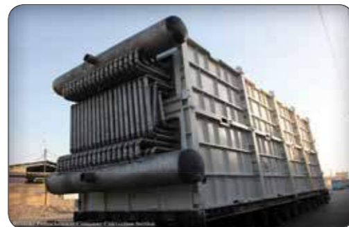
Bushehr Petrochemical Company convection section
