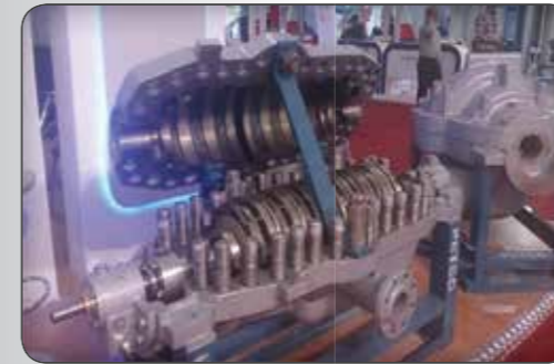
NISOC Project Pump Model: BS3-6x6 Capacity: 100 m 3 /h, Head: 370 m, Power: 200kw
