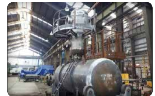
Deaerators And Water Softeners: Vertical And Horizontal Design With All Attachments, Including Internals, Ladder, Platform, External Jacket, Internal Coil
