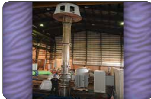
GHESHM Sea Water Intake Pump Type: VS1 Capacity: 2200 m 3 /h, Head: 70 m, Power: 630 kw
