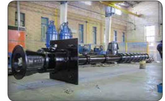
VS1 Pump With API-610 Standard
