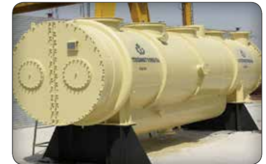
Surface Condenser (Esfahan Oil refinery)
