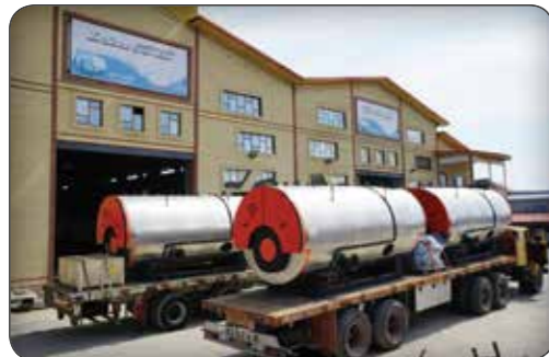
Atrin Parseh Greenhouse Uzbekistan Hot Water Boilers 4.500.000 K/Cal
