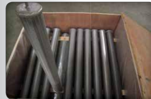
10- All types of cartridge filters up to 2 micron (Filters of Jam Petrochemical Co.)
