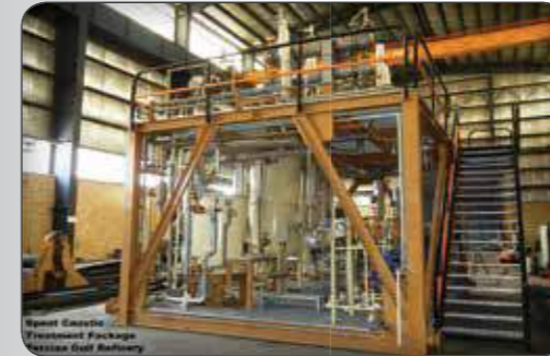
Spent Caustic Treatment Package Persian Gulf Star Refinery Client: Namvaran p&t (nardis-pgsoc)
