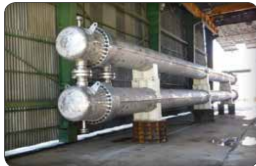
Shell & Tube Heat Exchangers (Manufacturing of Shell & Tube Heat Exchangers for Masjed Soleiman Petrochemical, Urea & Ammonia Plant)
