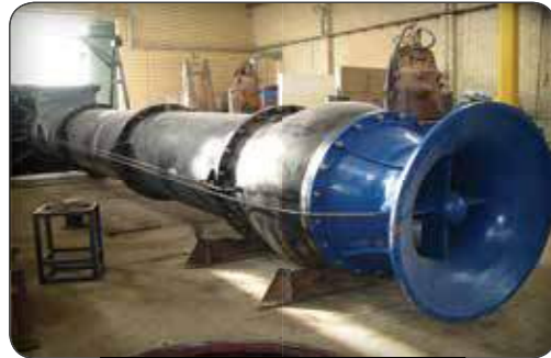
Submerged and sludge electro-pumps
