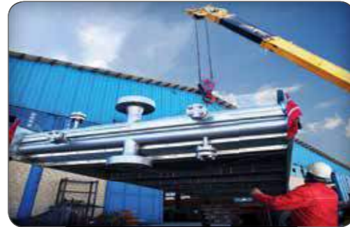
Air cooled Heat Exchanger ASME Sec VIII Div. 2 (Serajeh Gas injection Plant)
