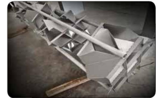
9- Static Mixers (Mixers of Bandar Abbas Oil Refinery Co.)
