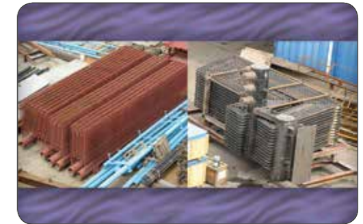
Super Heaters: ASME Sec1 up to 530 °C
