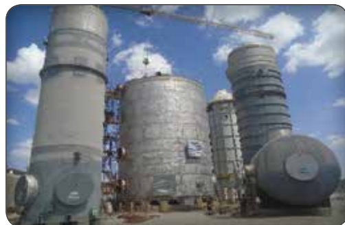
Converter & Heat Exchangers of Acid Plants Client.: Sarchesmeh & Katoon Abad Sulphuric Acid Plants.
