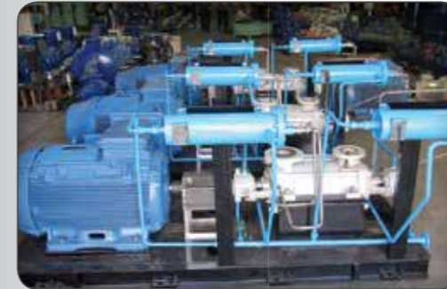
BB4 Pump With API-610 Standard
