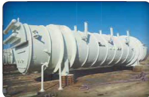
Indirect Heaters (Manufacturing of Indirect Heater for Haftkel Desalting Unit)
