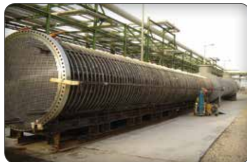
Shell & Tube Heat Exchanger.(AEL with Rod Baffles) Client.: Amir Kabir Petrochemical Company
