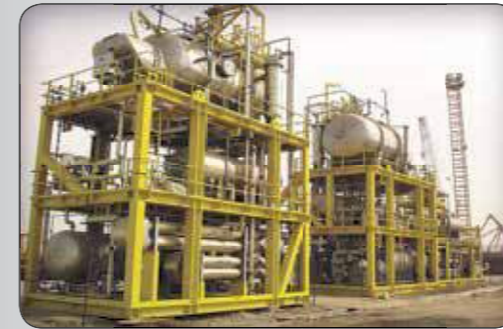
Process Packages & Skids ( Manufacturing of Gas Dehydration Package for Abuzar Oil Platform)
