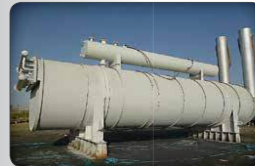
Heater – Ahwaz Desalting Plant - NISOC
