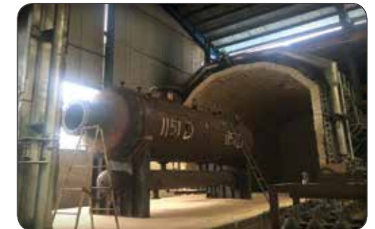
Makhzan Foolad Rafe Co. Iran – Mazandaran Normalizing, Annealing and Stress Relief Furnace Capacity 450 M3
