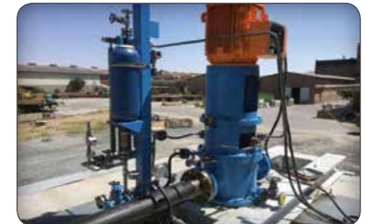
VS6 pump for Ilam SRU project in test stand
