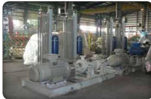
LAVAN Refinery Pump Type: BB5 Capacity: 25 m 3 /h, Head: 369.8 m, Power: 30kw
