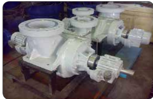
BB2 Pump With API-610 Standard
