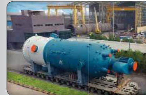
Marjan Methanol Plant Auto Thermal Reformer (ATR)
