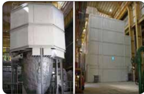
Construction of 94.2 Gas Turbine Enclosure units (Turbine Engineering & Manufacturing Company (TUGA))
