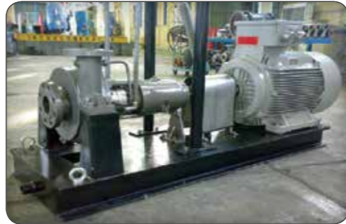
OH2 Pump With API-610 Standard
