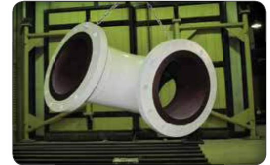
Custom Coating of Non-Tubular Products
