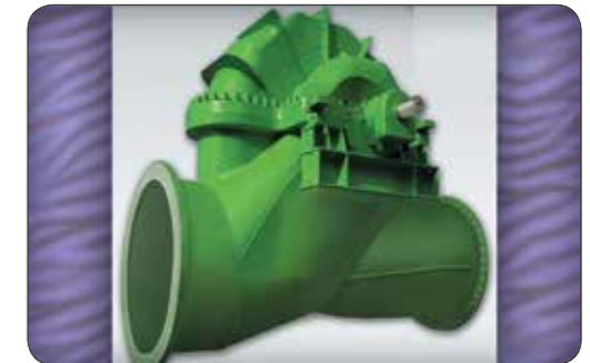
MAPNA Project, Cooling Power Plant Pump Type : 1200 DD 135 Capacity: 13700 m 3 /h, Head: 36 m, Power: 1.2 MW
