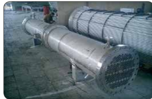
Heat Exchanger Fiber Intermediate Products Co. (DMT)
