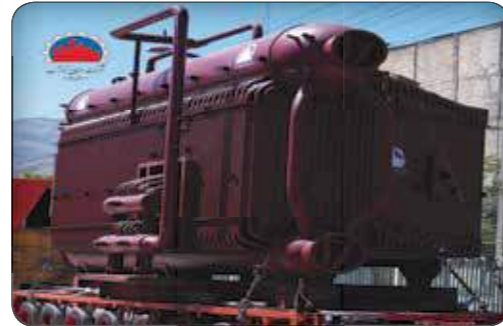
Water Tube Boiler Shahid Rajaie Power plant
